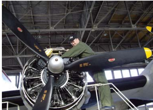
PARDON ME, GOVERNOR. Foundation Volunteer and A&P Mechanic Dan MacManus works on the #2 propeller governor.
