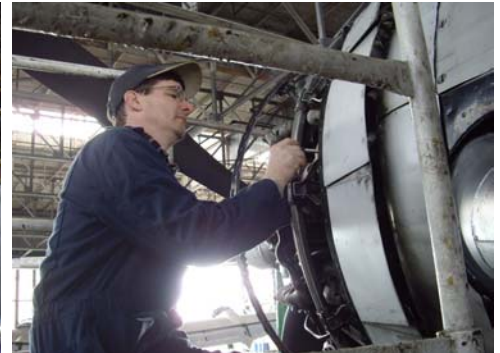
KEEPING IT COOL. Foundation Secretary Jeff DeKonty adjusts the cowl flaps on the #2 Engine.
