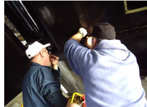
MONOTONOUS, ISN'T IT?. Foundation President and A&P Mechanic Tim Chopp works with Foundation Volunteer Steve Grubesich to remove over a hundred screws in order to access a fuel valve.
