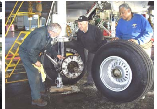
STOPPING POWER. Foundation Volunteers Frank Benson and Cedric Morrison and A&P Mechanic Joe Tesoriero inspect one of the C-54's 4 brakes.
