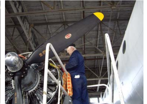
MAKING ADJUSTMENTS. Foundation Volunteer Jim Reed works to adjust the cowl flaps on the #3 engine of the C-54.
