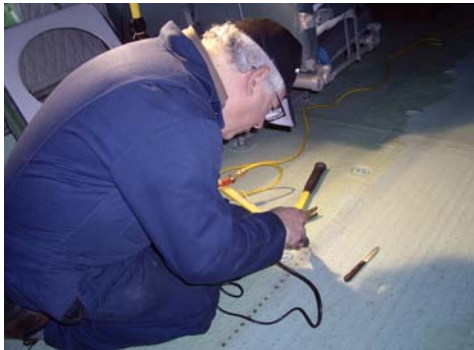
FLOORED. Foundation Volunteer Art Kunhardt removing the cabin floor access panel for an inspection
