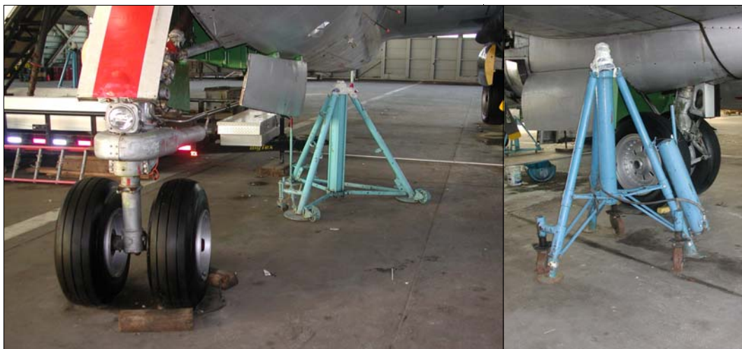
TWO OF THREE JACKS PURCHASED BY THE FOUNDATION IN OCTOBER 2004. EACH JACK HAS THE CAPABILITY OF LIFTING 30 TONS. THESE JACKS CAN BE USED ON THE C-54 AS WELL AS THE C-97.
