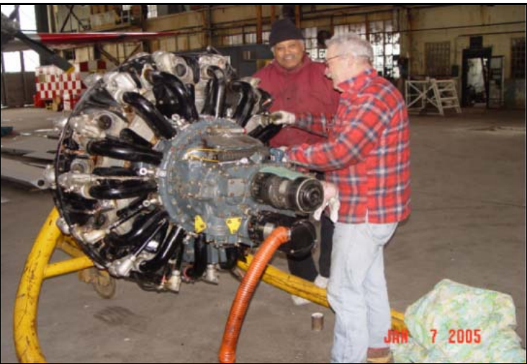
Foundation Volunteers (L to R) Cedric Morrison and Ray Keating help prepare a replacement Pratt & Whitney R-2000 engine for installation on the C-54, "SPIRIT OF FREEDOM"
