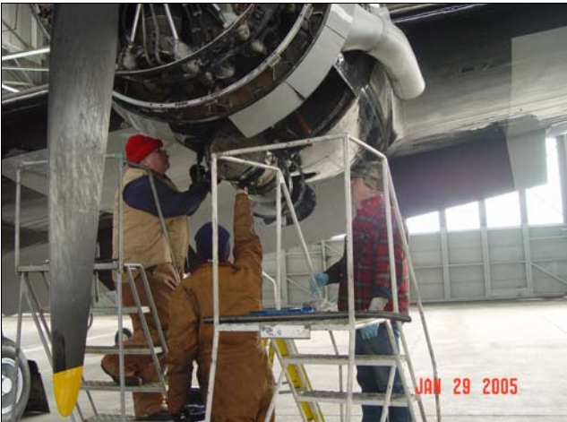
Foundation Maintenance Volunteers Michael Shay, A&P Mechanic Dan McManus, and Ray Keating remove an oil cooler from the C-54 "Spirit of Freedom"
