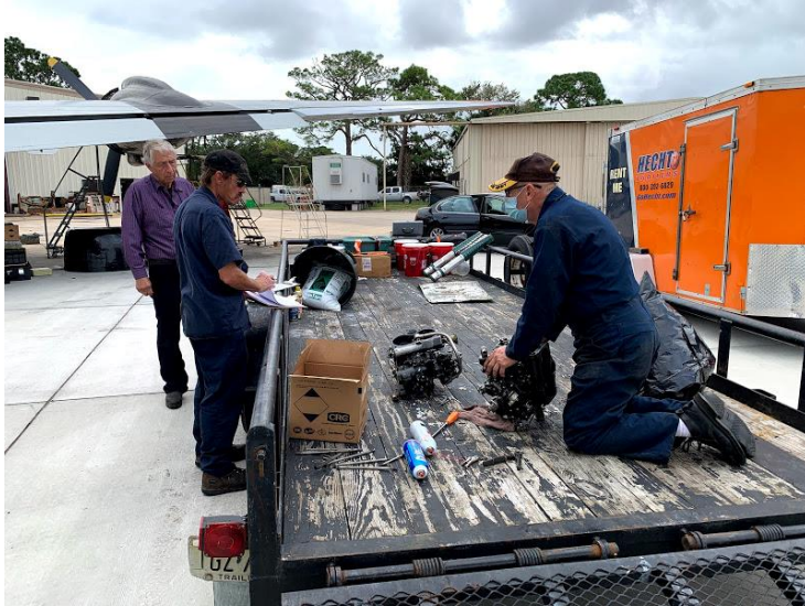
TIM CHOPP INSPECTING THE CARBURETOR OFF THE # 4 ENGINE WHILE JASON PENCE CHECKS OFF THE INSPECTION INSTRUCTIONS. JIM REUGER IS OBSERVING THE PROCEDURE. TIM MAKES THE DRIVE TO NEW SMYRNA BEACH FROM NEW JERSEY. JASON MAKES THE DRIVE FROM WOODSTOCK, VA, AND JIM MAKES THE DRIVE FROM TOLEDO, OHIO. THIS IS THE 4TH VISIT FOR ALL THREE MEN TO INSPECT AND REPAIR OUR REPLACEMENT C-54D.
