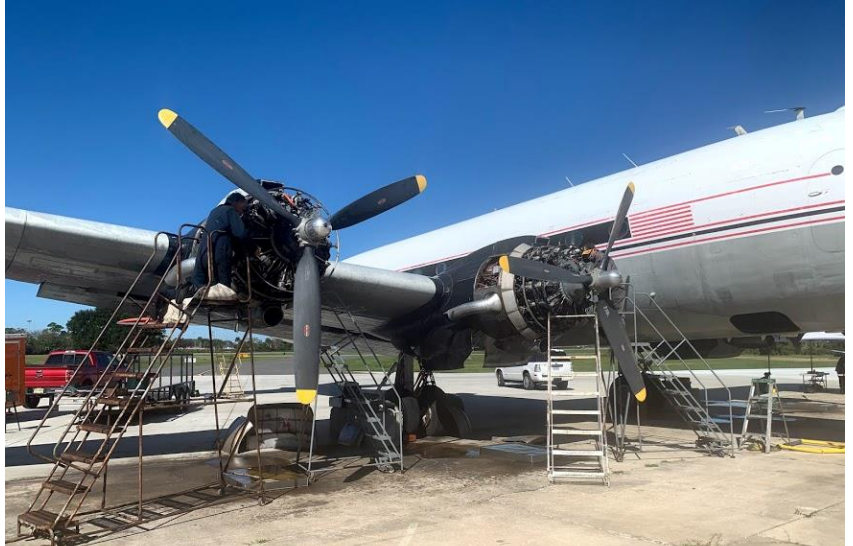
NOVEMBER 2020: DOUGLAS C-54D 43-17228 BEING INSPECTED AT NEW SMYRNA BEACH, FL. TIM CHOPP REPLACING THE LEFT MAGNETO ON THE # 3 ENGINE WHILE JIM REUGER INSTALLS SPARKPLUGS ON THE # 4 ENGINE.
