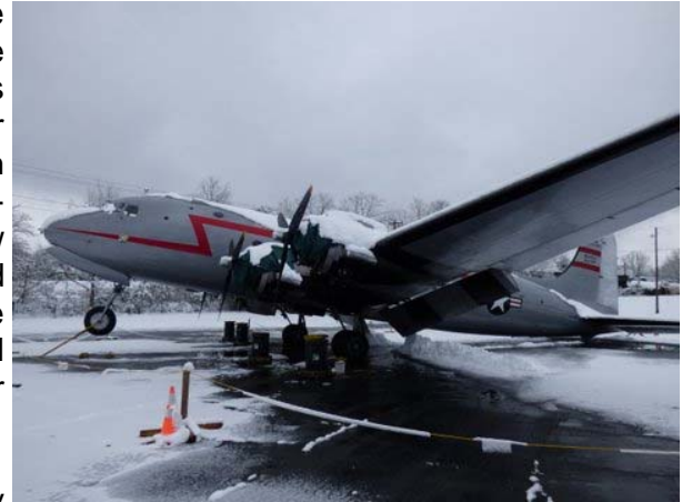
THE HAZARDS OF NOT BEING IN A HANGAR FOR THE WINTER. THE "SPIRIT" SETTLES ON ITS TAIL SKID BY THE WEIGHT OF THE SNOW. NO DAMAGE WAS DONE AS A RESULT OF THIS.
