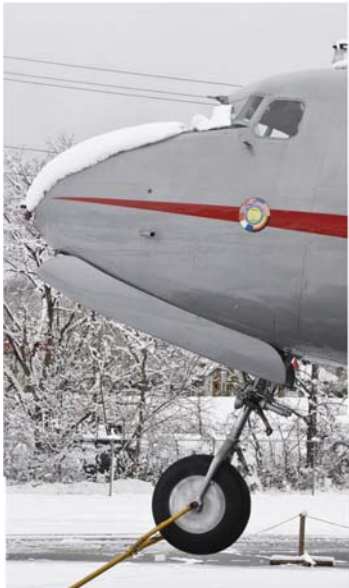
NOSE HIGH ATTITUDE: THE C-54 NOSE WHEEL ABOUT 3 FEET OFF THE GROUND AS A RESULT OF THE SNOW WEIGHTED TAIL AFTER A STORM IN WINSTON SALEM NC.
