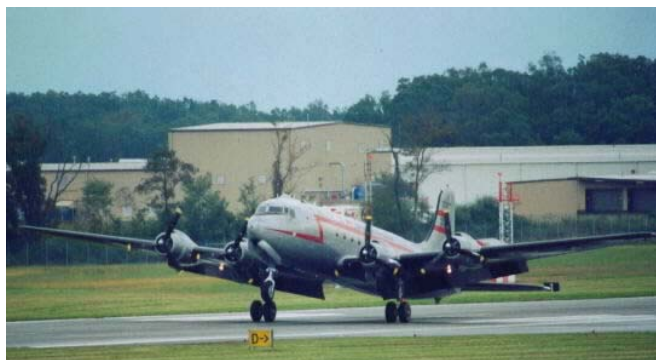
The "Spirit of Freedom" using a nose high attitude for aerodynamic braking to reduce the landing distance and wear on the wheel brakes.
