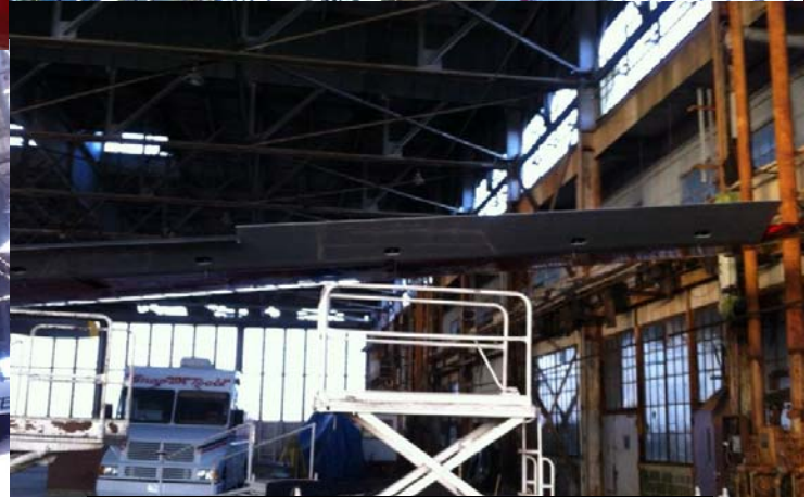
The newly recovered right aileron has been installed on the C-97.
