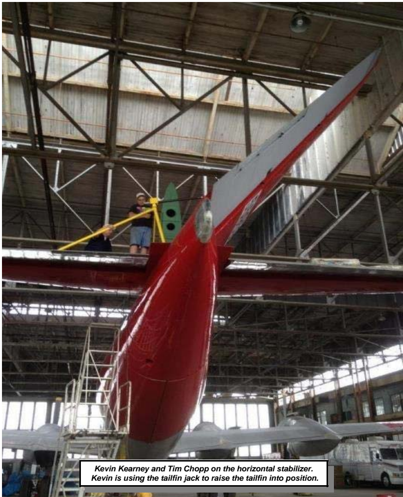
The C-97 tail in flight position. It will have to be lowered again in order to get the airplane out of the hangar, but the jacking procedure works like a charm.
