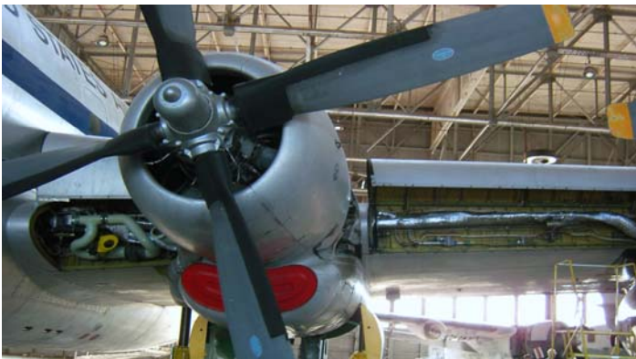
The wing leading edges have all been opened and the wings and systems have been inspected and the areas all cleaned up.
